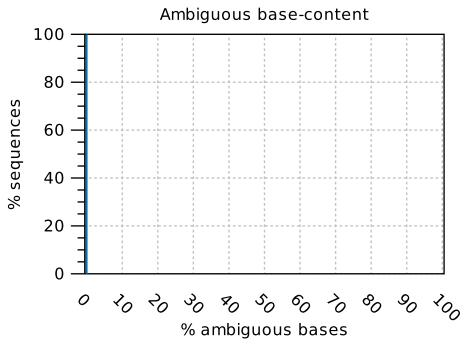
Distribution of N-contents. The N-content of a sequence is calculated as the number of amb iguous bases compared to all bases.
